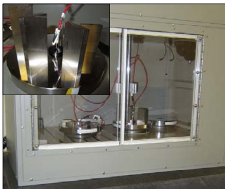
Figure 1. Laser interferometer measuring chamber for calibration GB (NPL TESA AGI 300 – Czech metrological institute)
