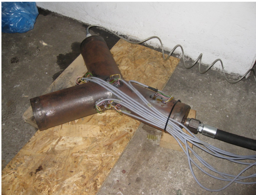
Figure 3. Strain gauges on the experimental Y-shape branch (MM - measuring point)
