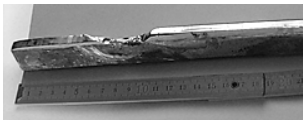
a) catastrophically damaged knife
