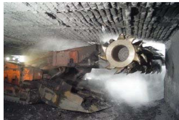
Figure 2. Cutting action of continuous miner machine
