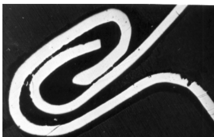
Figure 13 Lid of the tin damaged by corrosion
