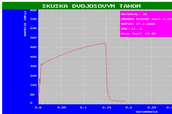
Figure 1 T Dependence stress-strain of material TH 435 CA, thickness 0.24 mm
