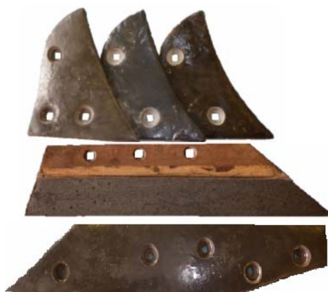
Figure 8. Prototypes of exchangeable parts of moldboard and land side with composite layer (F60, F80 a F240)
