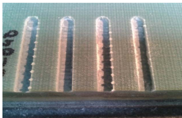
Figure 9. Created grooves to material GFRP [1]
