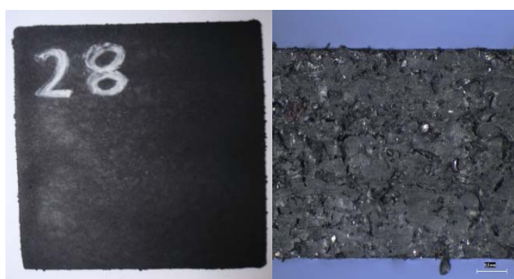
Figure 6. Moulding with p = 230 bar, \vartheta = 230^\circ\text{C} , m = 42 g, t = 25 min
