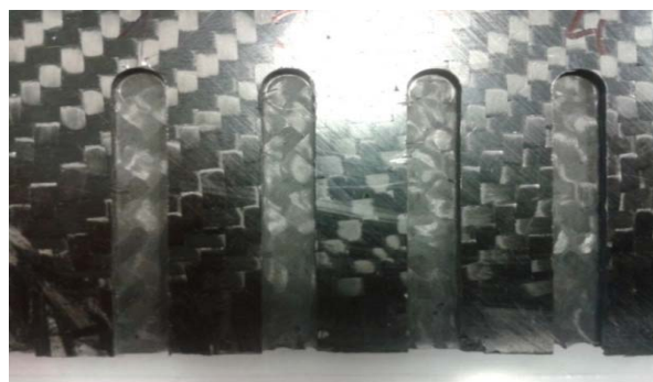
Figure 10. Created groove at CFRP [1]
