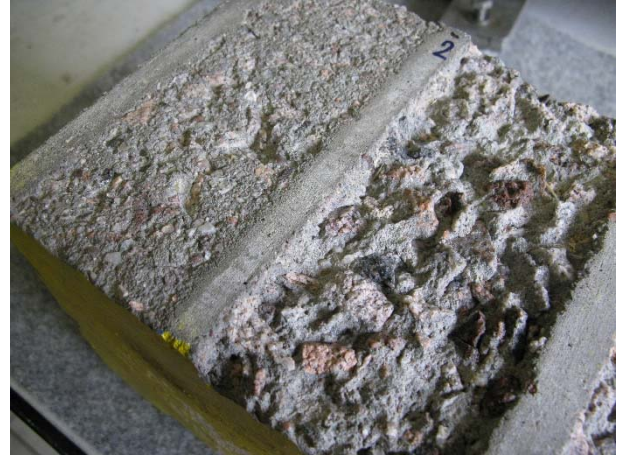
Figure 4. Example of surfaces created by three passes (side by side) of both flat continuous (left) and flat pulsating (right) jets on concrete sample (water pressure 30 MPa, equivalent nozzle diameter 2.05 mm, stand off distance 40 mm, traversing velocity 0.2 \text{ m.min}^{-1} )
