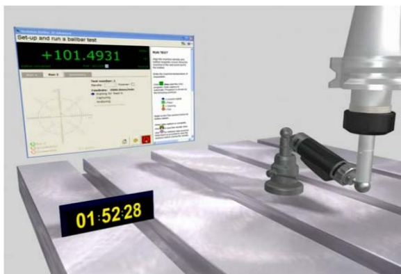
Figure 7. Testing by QC20-W ballbar with new function including of a partial arc
