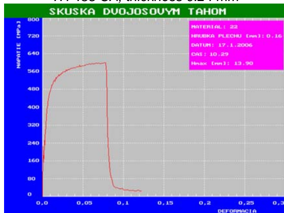
Figure 2 T Dependence stress-strain of material TS 550 BA, thickness 0.16 mm
