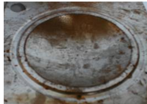
Figure 7 Sheet TS 550 BA after breakage
