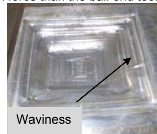
Fig7. Formation of wave using conical end tool
