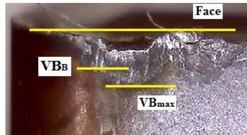
Figure 7. Wear of inserts - CNMG 120408 - M5
