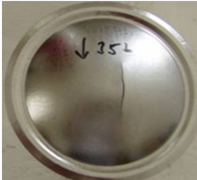
Figure 10 Sheet TH 435 CA after breakage before corrosion
