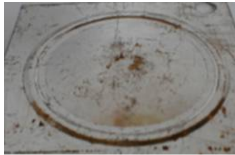
Figure 4 Sheet TH 435 CA after 5% deformation
