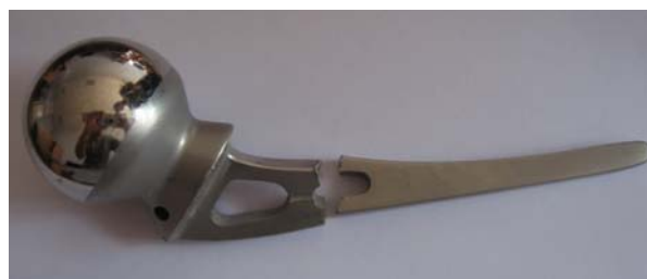
Figure 1. Artificial hip prosthesis failure
