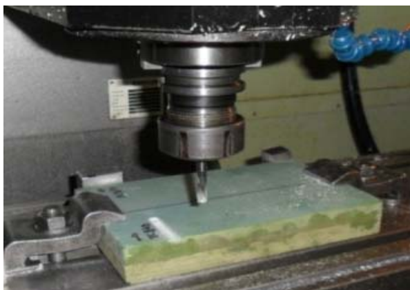
Figure 8. Cutting of grooves to material GFRP [1] Experimental results are presented in following tables:
