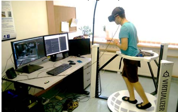
Figure 2. Combination of VR tools – Walking in the virtual assembly shop
