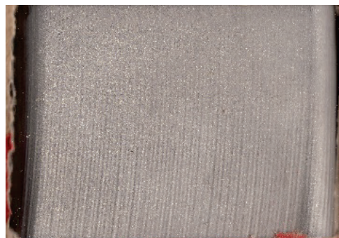
Figure 2. Surface sample after abrasive jet cutting of stainless steel
