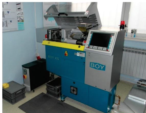
Figure 1. Injection molding machine installed at Mechanical engineering faculty in Slavonski Brod
