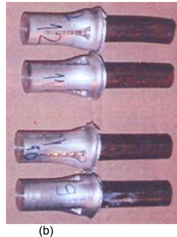
Figure 2. Technical drawing and physical appearance of samples (a) and welded Al-Cu samples (b)
