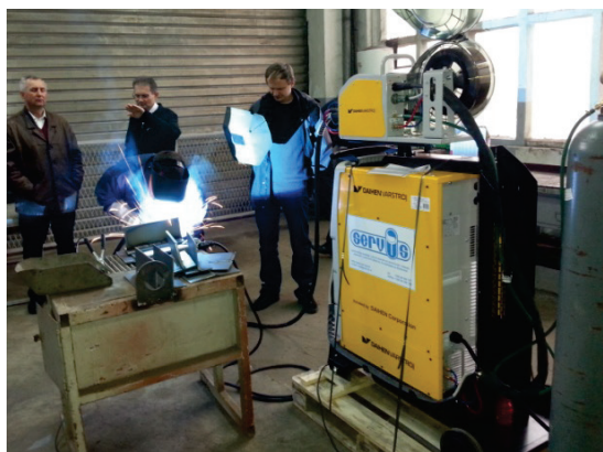
Figure 3. Welding with the device for welding Welbee P500L
