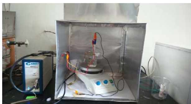
Figure 2. Faraday cage with system of electrodes
