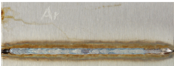
Figure 7. Corrosion attack of sample Ar2 (weld surface)
