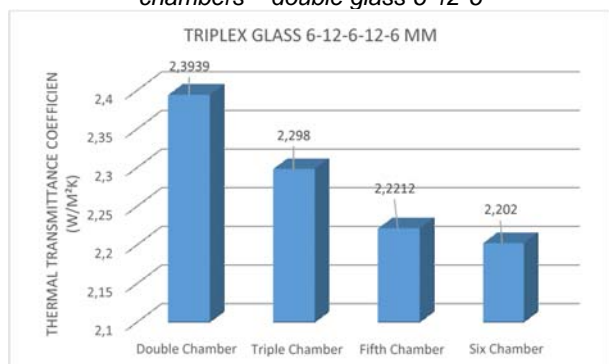
Figure 4. Heat transfer coefficient ( W/m^2K ) for transparent element "9", Tab. 1 for different number of chambers – triple glass 6-12-6-12-6 mm
