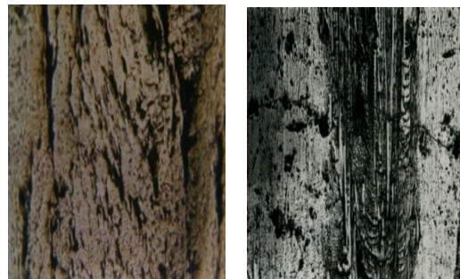
Figure 2. Area damaged by adhesion [1]
