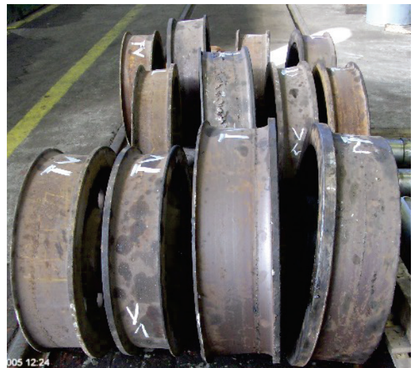
Figure 5. Wheel damage due to rim wear
