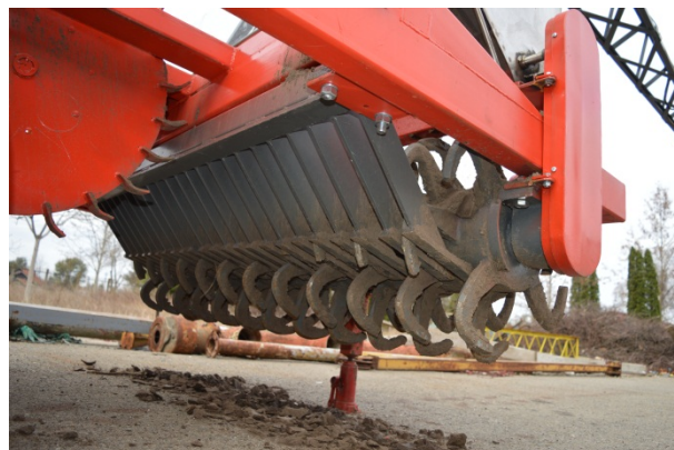
Figure 3. Cylindrical roller with specially shape teeth
