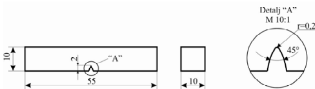
Figure 3. Test specimen for Charpy impact test
