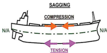
Figure 14a). Schematic representation when the ship is on the crest of wave
