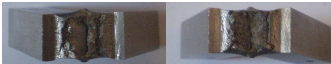
Figure 11. Appearance of fracture surfaces of the specimen for impact testing
