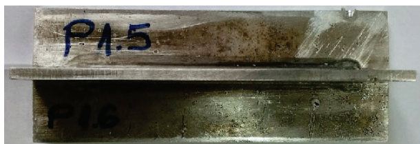
Figure 5. Root side of T joint of AA 5052-H32
