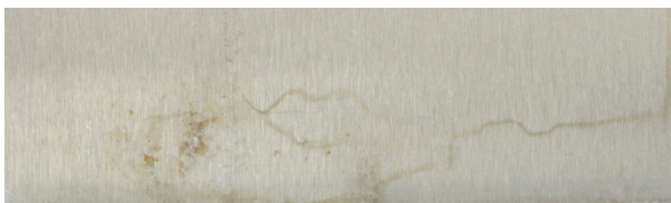
Figure 6. Corrosion attack of base material
