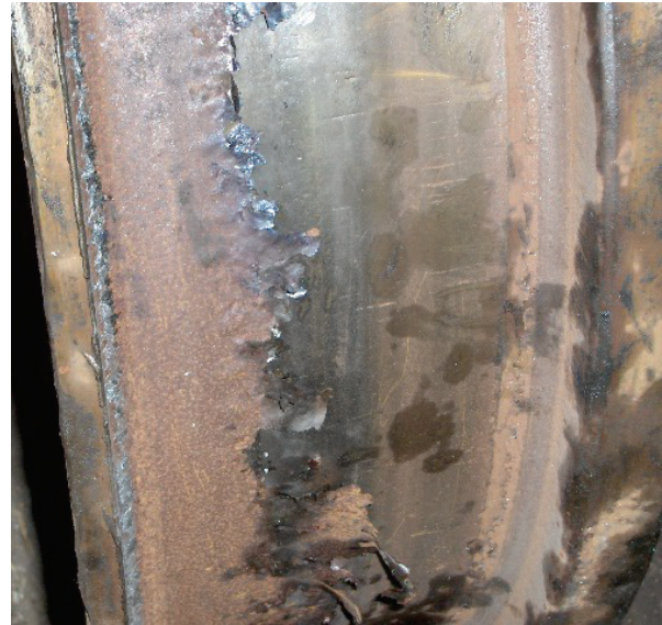
Figure 4. Wheel damage due to drift surface wear
