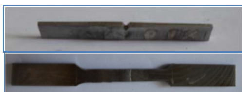
Figure 2. Charpy and tensile specimens [6-8].
