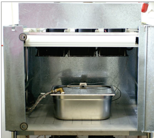
Figure 1. Artificial aging equipment fitted with water basin
