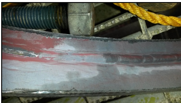
Figure 3: Segments of the 50 mm wide old weld revealing root defects
