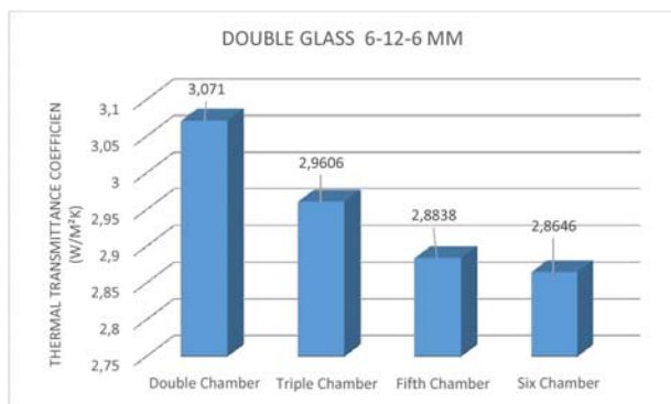
Figure 3. Heat transfer coefficient ( W/m^2K ) for transparent element "9", Tab. 1 for different number of chambers – double glass 6-12-6
