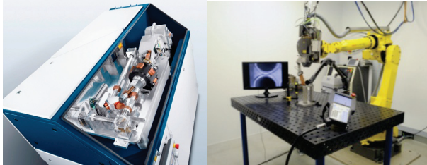
Figure 4. TRUMPF TruDisk 4002 laser device (left), Fanuc M-710iC/50 robotic arm (right)
