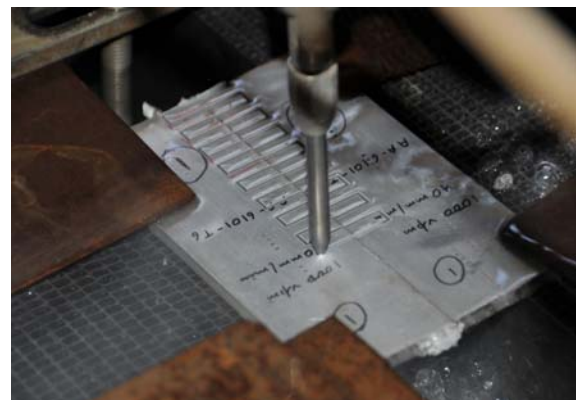
Fig. 4 Progress of Comb profile Water Jet Cutting of Friction Stir Welded Aluminium Plates
