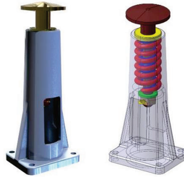
Figure 6. Mounted composition of the damper
