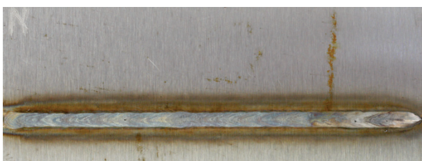
Figure 9. Corrosion attack of sample N1 (weld surface)
