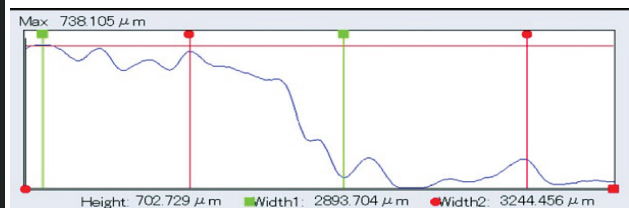
Figure 6. The 3D profile of fracture surface of Charpy specimen 2 (20°C).
