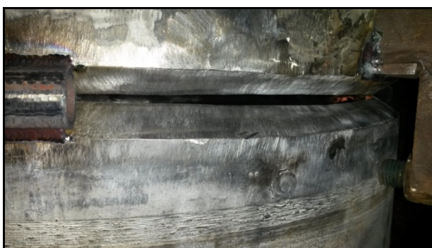
Figure 5: Fit up and tack welding
