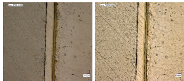
Figure 6. Microstructure of weld joint interface AI7075/Ag/AZ31B
